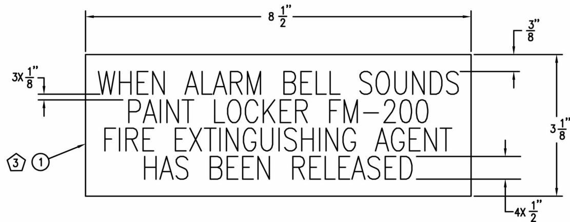
VIEW 14-C PAINT LOCKER FM-200 SYSTEM ALARM BELL LABEL PLATE
