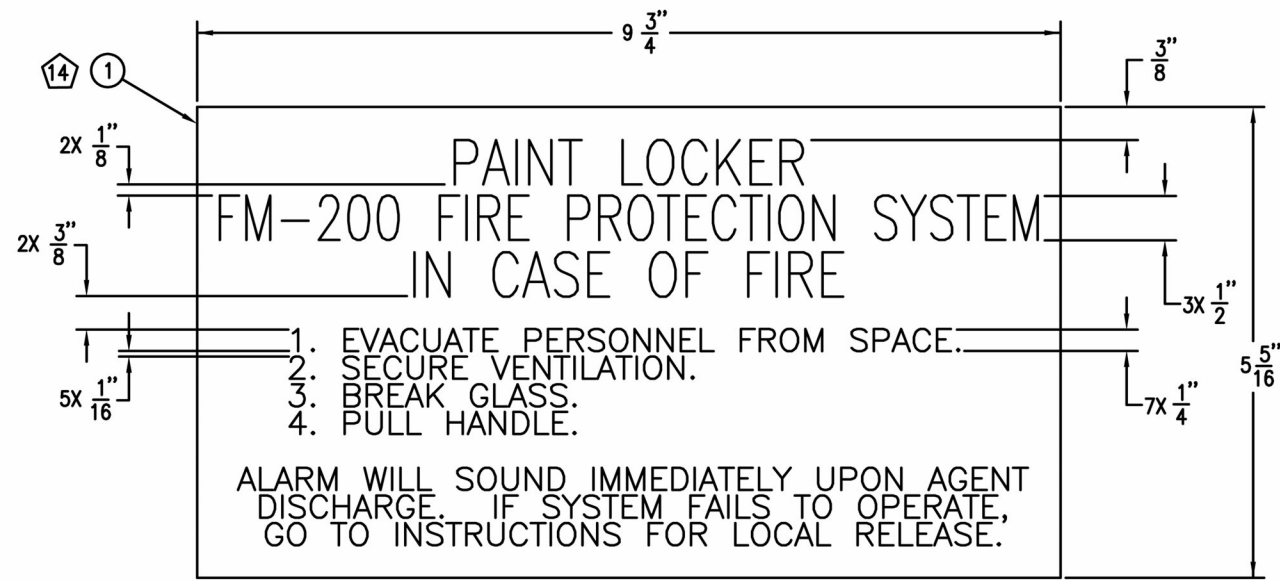
VIEW 30-C PAINT LOCKER FM-200 SYSTEM REMOTE OPERATION INSTRUCTION PLATE
